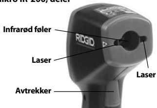
Figur 2 – mikro IR-200, deler
